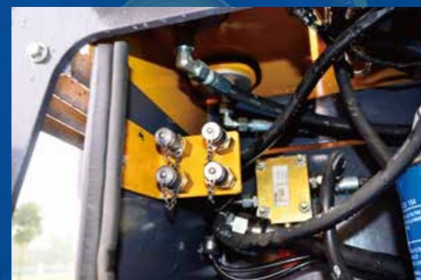
Centralized pressure measurement
